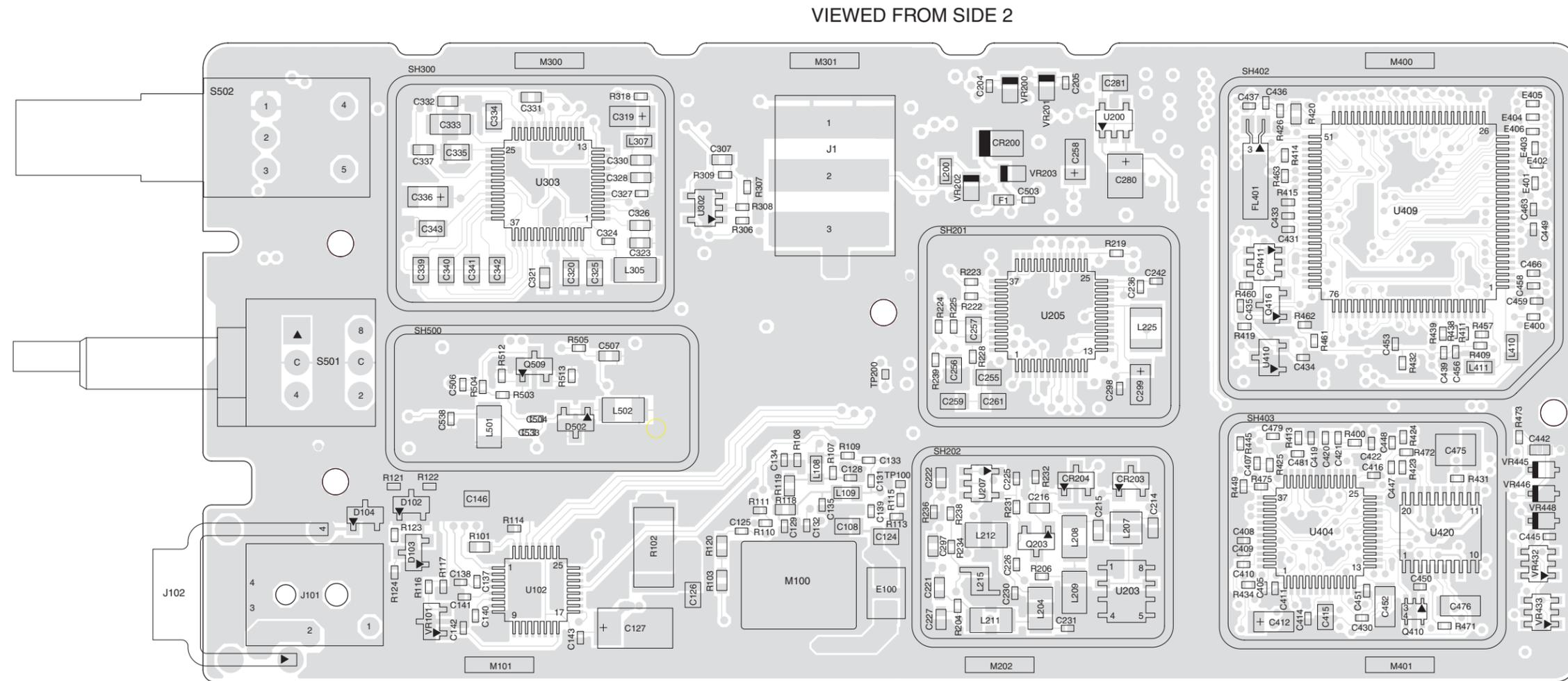
Figure 4-81: Low Band (29.7-42/35-50 MHz) Main Board Bottom Side PCB
